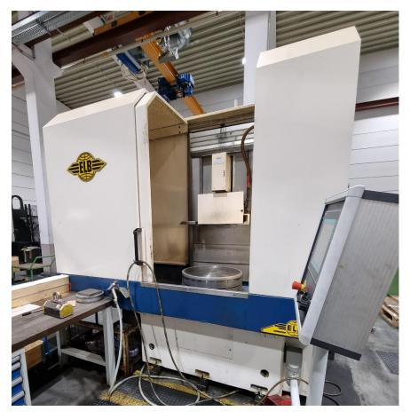
High Quality horizontal flat grinding machine with automatic dressing unit, rotary table, big vertical travel and full enclosure.
